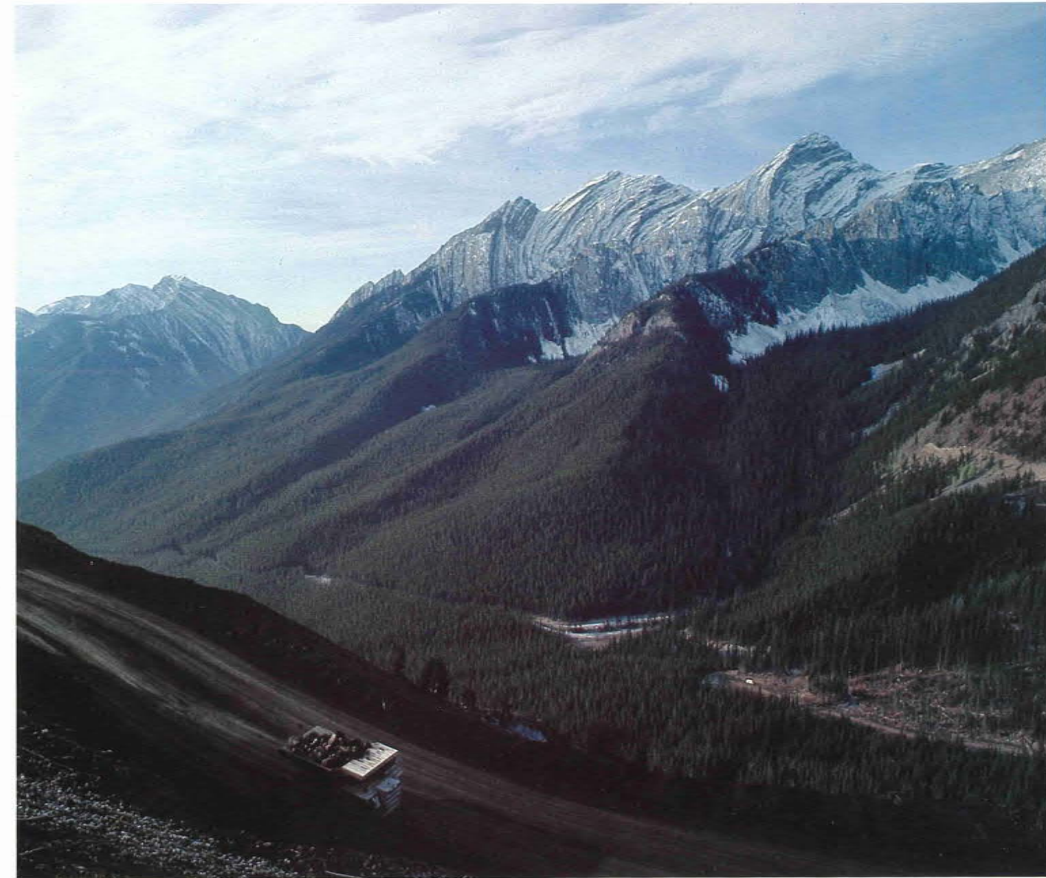
▲► The open pit mine is located high in the mountains atop Line Creek Ridge where waste rock is removed to expose the coal seams and hauled to the adjacent valley.
