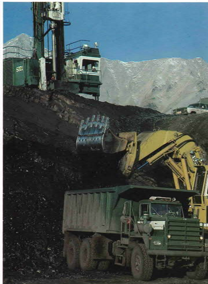
▲ Coal is loaded by hydraulic excavators for transport to the preparation plant.
