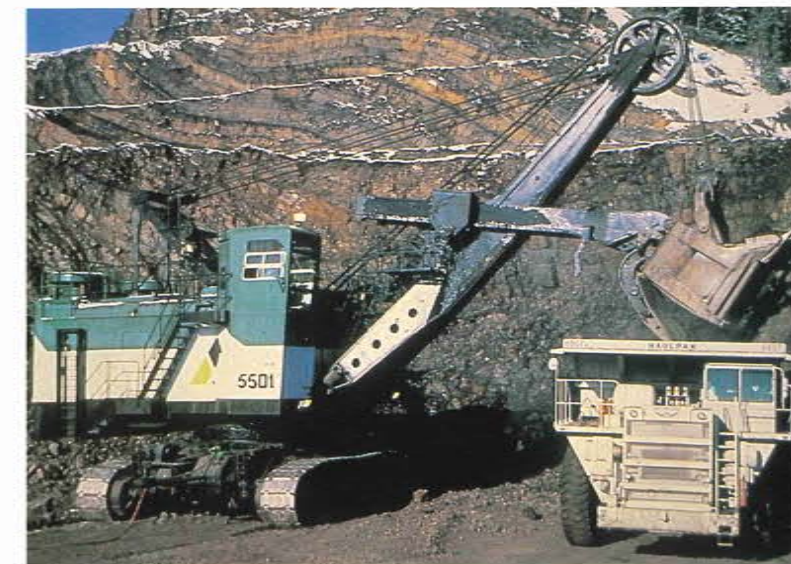
▲► The open pit mine is located high in the mountains atop Line Creek Ridge where waste rock is removed to expose the coal seams and hauled to the adjacent valley.
